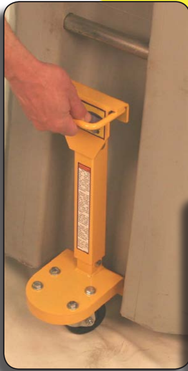
Hook the bottom edge on the container
