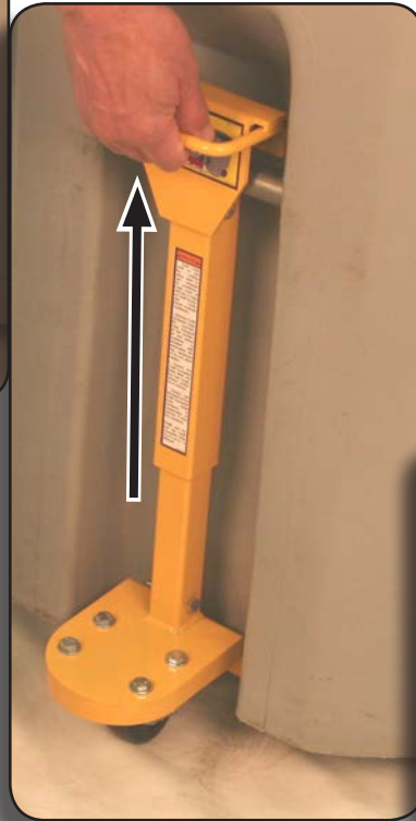
Hook the cross bar on the container
