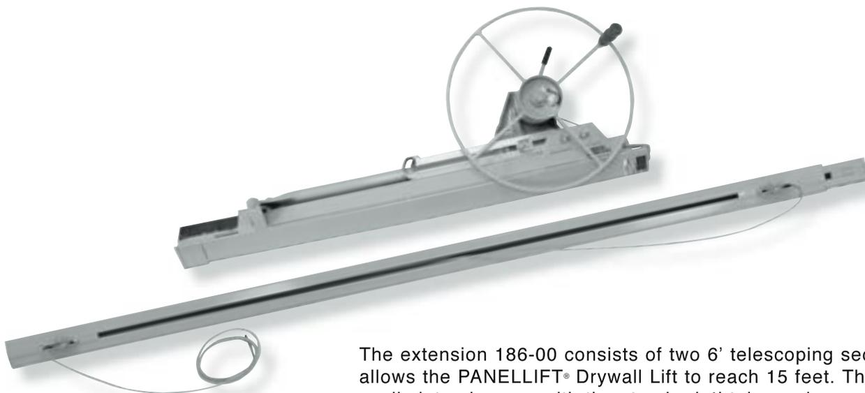
The extension 186-00 consists of two 6' telescoping sections and allows the PANELLIFT® Drywall Lift to reach 15 feet. This unit easily interchanges with the standard 4' telescoping sections of the PANELLIFT® Model 138-2 shown here for comparison.
