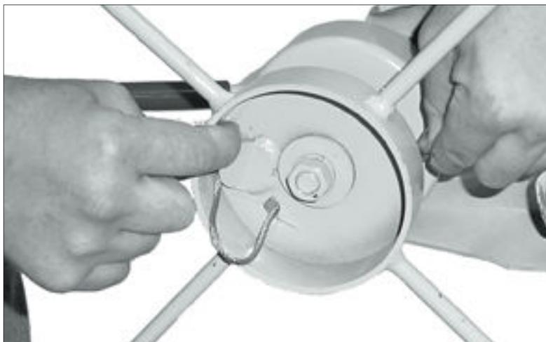
1. Loosen the cable from the mooring tab on the winch and pull it out from the winch drum. **BE CAREFUL!** A worn cable can have frayed strands. Wearing gloves will help protect your hands.
