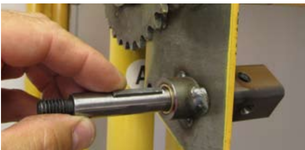
13) Install the key in the slot of the shaft
