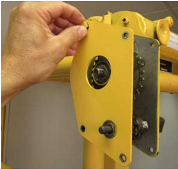
15) Install the outer hanger bracket by starting the single 1/4" x 2 1/2" bolt in the uppermost hole as shown. DO NOT fully tighten this bolt at this time. (Wait until step 19 below.)
